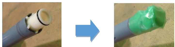
Figure 4-4 Example of covered top of collecting pipe
